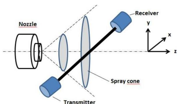
**Figure 2.** Schematic of the droplet size measurement setup
