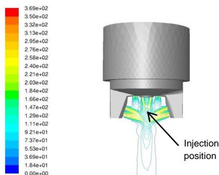
Figure 9. Velocity contours near the atomizer
