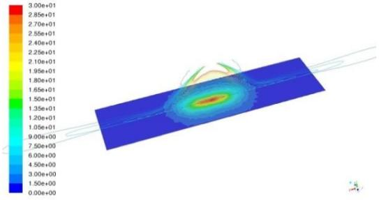
**Figure 13.** Calculated velocity contours colored by velocity magnitude [m/s] in the cross-section  $z = 0$  with hexahedral mesh model without atomizer. The static film thickness distribution on the plate is also overlaid.
