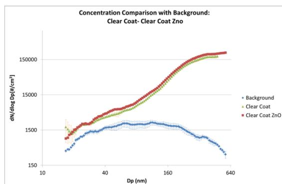
**Figure 7.** Clear coat particle concentration at the measuring position: L50cm, W0, H79.5cm
